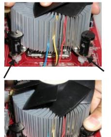
7. Align the fastener tips with the motherboard hole pattern, insert the fastener tips into the holes, guiding the wires to avoid pinching. The fasteners will slide through the motherboard holes with no insertion force.
