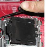
4.Use index finger and thumb to press down metal lever, the cap will be pushed up by the CPU; this may also be done by removing the cap beforehand.
