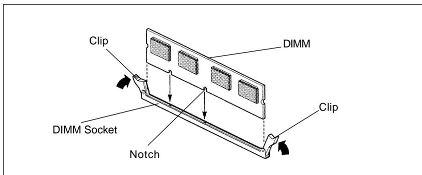
5. Position the DIMM above the socket. Align the two small notches in the bottom edge of the DIMM with the keys in the socket.
