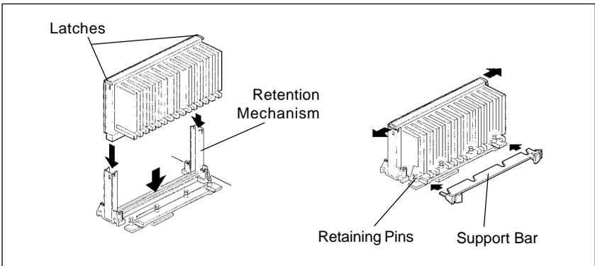
3. Slide the top heatsink support bar onto the retaining pins of the support's base as shown in figure.
