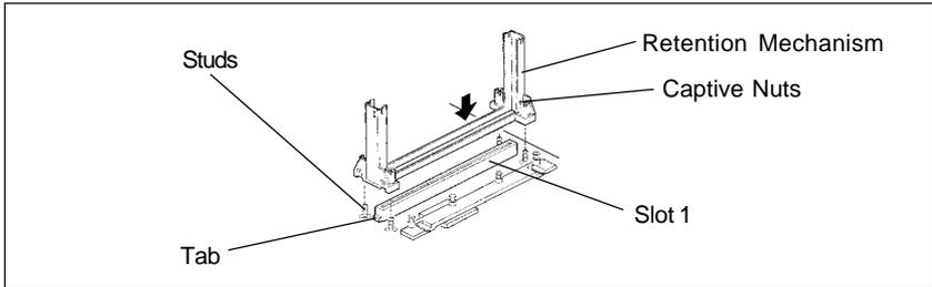
3. Finger tighten all four captive nuts to make sure they start correctly on the threads of the attachment studs.
