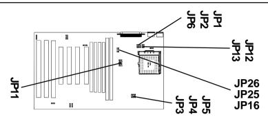
JP11, JP12, JP13, JP16 - Power Selection for the CPU Bus Section, Bus Voltage & CPU Core-Voltage Select
