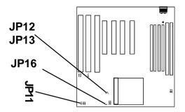
JP11, JP12, JP13, P16 - Power Selection for the CPU Bus Section, Bus Voltage & CPU Core-Voltage Select
