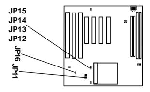
JP11, JP12, JP13, JP14, JP15, JP16 - Power Selection for the CPU Core Voltage, Bus Section and Bus Voltage
