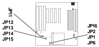
JP11, JP12, JP13, JP14, JP15, JP16 - Power Selection for the CPU Bus Section, Bus Voltage & CPU Core-Voltage Select
