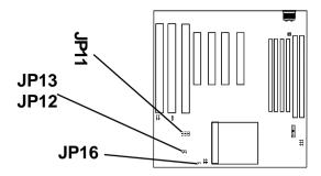
JP11, JP12, JP13, P16 - Power Selection for the CPU Bus Section, Bus Voltage & CPU Core-Voltage Select
