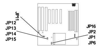
JP11, JP12, JP13, JP14, JP15, JP16 - Power Selection for the CPU Bus Section, Bus Voltage & CPU Core-Voltage Select
