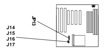
JP13, J14, J15, J16, J17- Power Selection for the CPU Bus Section & CPU Core-Voltage Select
