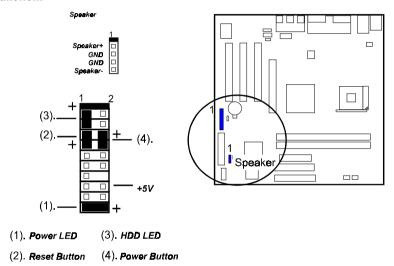
**Power LED** is connected with the system power indicator to indicate whether the system is on/off. It will blink when the system enters suspend mode.
