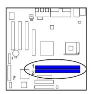
Press the clips with both hands to remove the DIMM.
