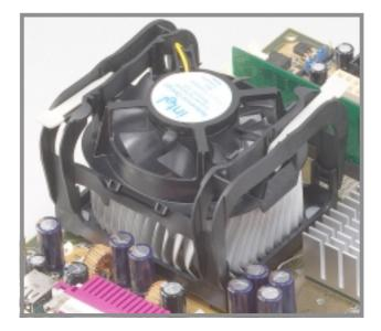
4. Connect the CPU fan cable. With the fan, heatsink, and the retention mechanism in place, attach the CPU fan cable to the connector on the motherboard labelled CPUFAN
