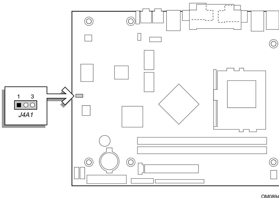
**Figure 9. Location of the BIOS Setup Jumper Block**
