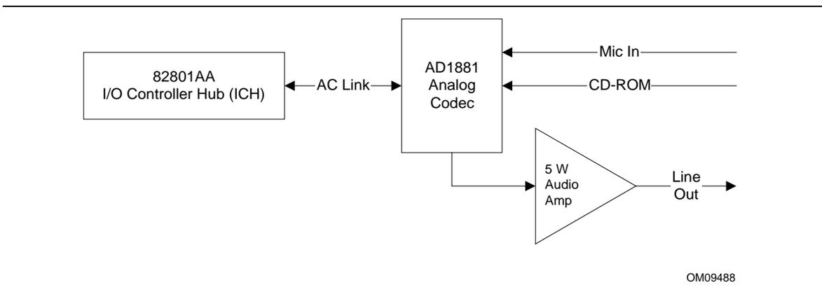
**Figure 4. Block Diagram of Audio Subsystem with AD1881 Codec**
