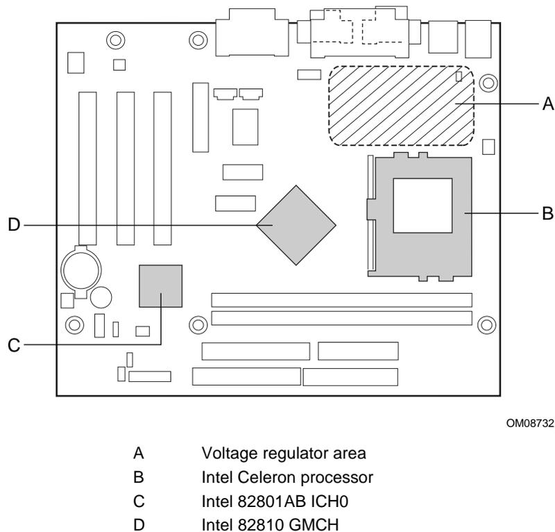
**Figure 15. Thermally-sensitive Components**
