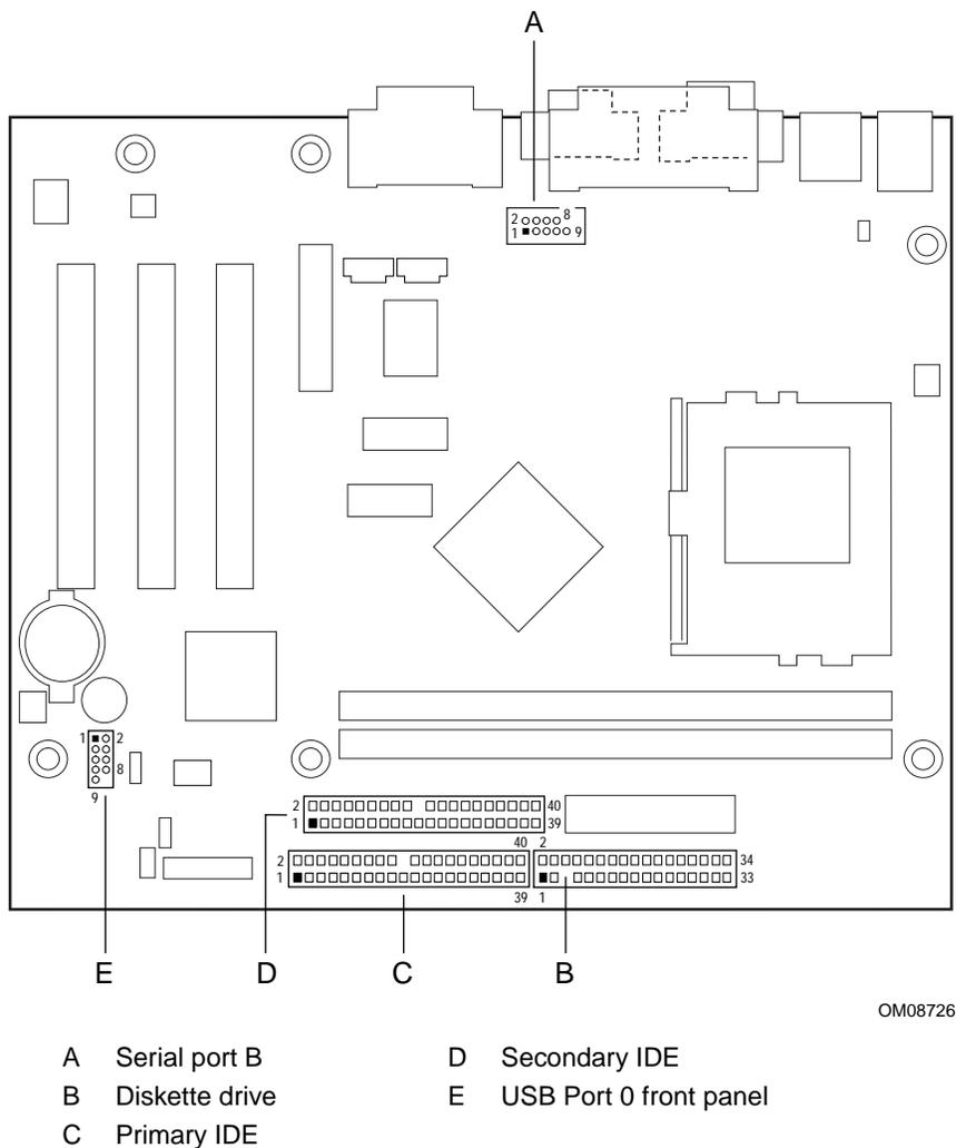
**Figure 8. Peripheral Interface Connectors**
