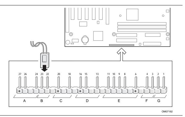
Figure 6. Front Panel I/O Connectors
