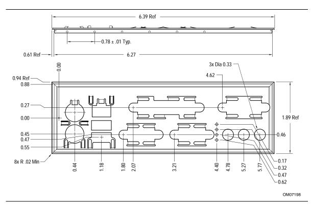
Figure 11. Back Panel I/O Shield for Motherboards with Extended Diagnostics Option (ATX Chassis Independent)
