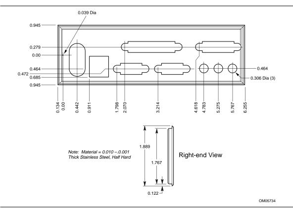
Figure 10. Back Panel I/O Shield Dimensions (ATX Chassis Independent)
