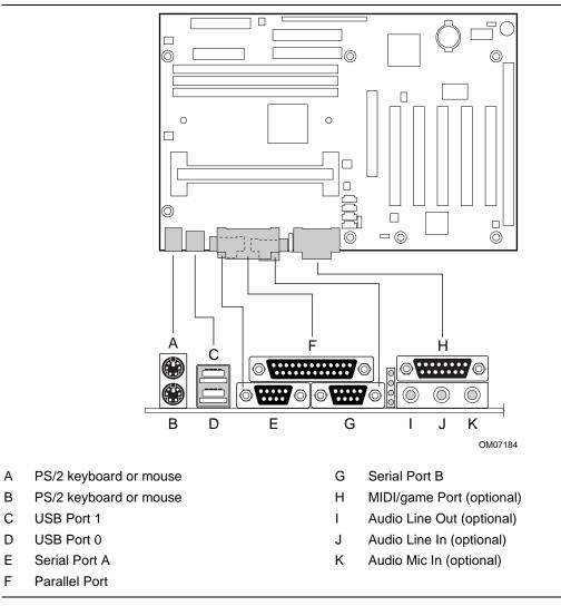
Figure 4. Back Panel Connectors
