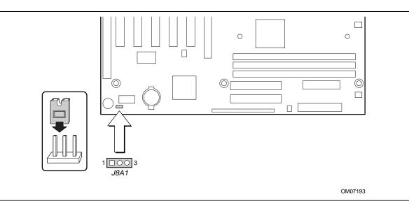
Figure 7. Location of the Configuration Jumper Block
