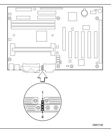
Figure 2. Diagnostic LEDs
