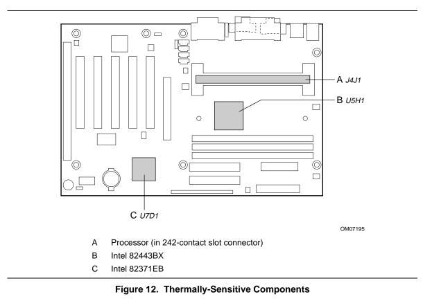
Figure 12 shows motherboard components that may be sensitive to thermal changes.
