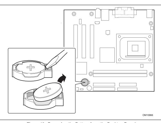
Figure 10. Removing the Battery from the Desktop Board
