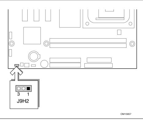
Figure 9. Location of the BIOS Configuration Jumper Block
