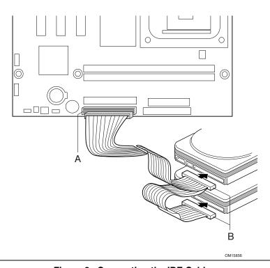
Figure 8. Connecting the IDE Cable
