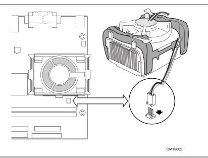
Figure 6. Connecting the Processor Fan Heatsink Cable to the Processor Fan Header
