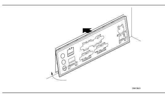
Figure 3. Installing the I/O Shield
