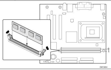
Figure 7. Installing Memory
