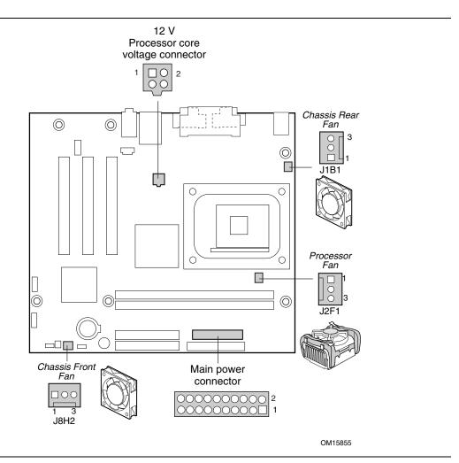
Figure 13. Fan Headers and Power Connectors
