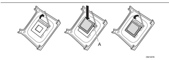
Figure 5. Installing a Processor
