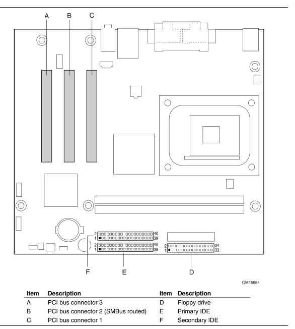
Figure 14. Add-in Card and Peripheral Interface Connectors
