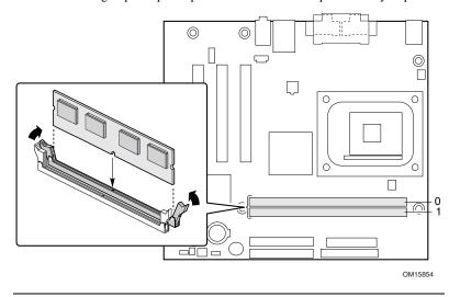
Figure 4. Installing a Memory Module
