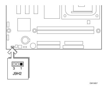
Figure 8. Location of the BIOS Configuration Jumper Block
