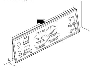
Figure 2. I/O Shield
