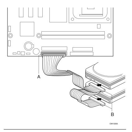
Figure 5. Connecting the IDE Cable
