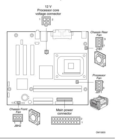
Figure 7. Location of Fan Headers and Power Connectors
