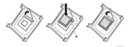
Figure 3. Installing the Processor
