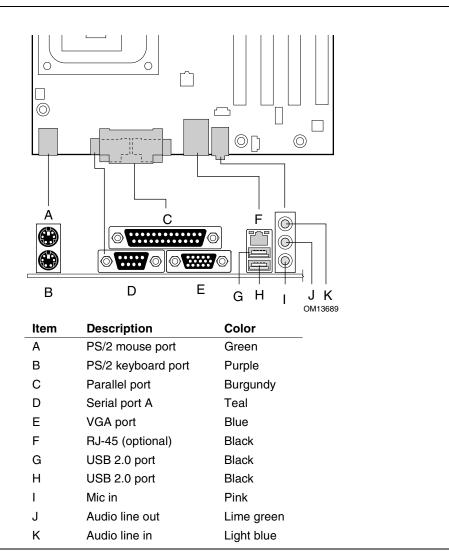
Figure 12. Back Panel Connectors
