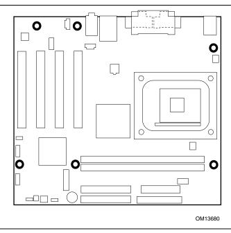
Figure 4. Desktop Board Mounting Holes
