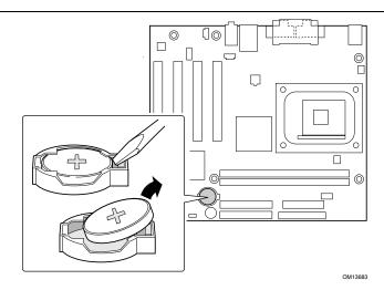
Figure 11. Removing the Battery from Desktop Board D845GLLY
