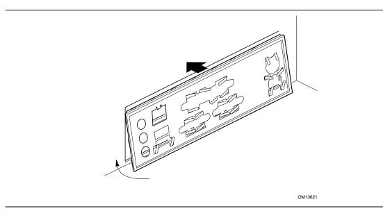
Figure 3. Installing the I/O Shield
