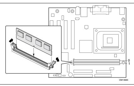
Figure 7. Installing a DDR SDRAM DIMM
