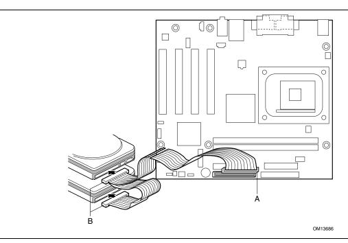
Figure 8. Connecting the IDE Cable
