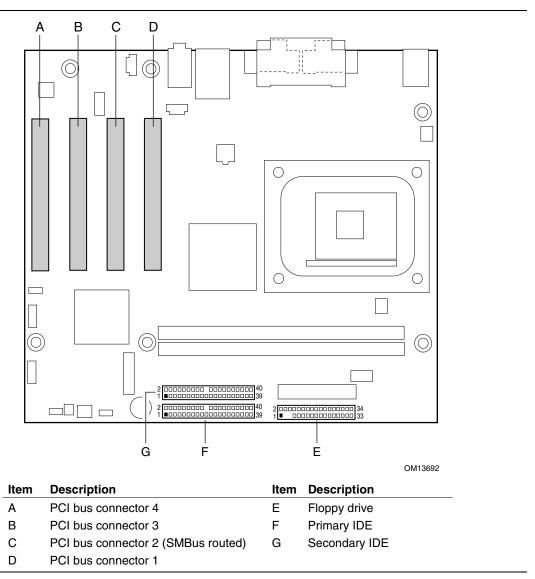
Figure 15. Add-in Card and Peripheral Interface Connectors
