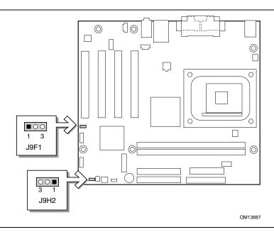
Figure 9. Location of the BIOS (J9H2) and Front Panel USB Wake Configuration (J9F1) Jumper Blocks
