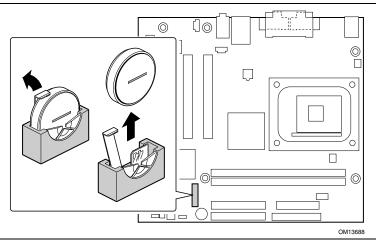
Figure 10. Removing the Battery from Desktop Board D845GLAD
