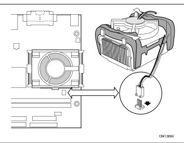
Figure 6. Connecting the Processor Fan Heat Sink Cable to the Processor Fan Connector
