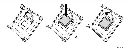
Figure 5. Installing a Processor
