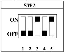
**P54C STD:** 3.135V ~ 3.600V (The fourth line of the mark on the under-side of the processor contains a code that identifies the voltage level type. V is VRE, S is standard.)
