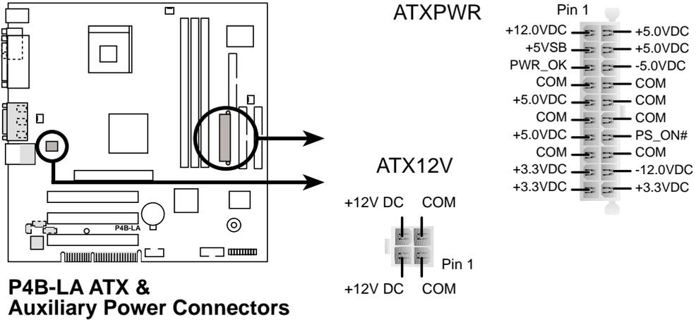
**P4B-LA ATX & Auxiliary Power Connectors**
