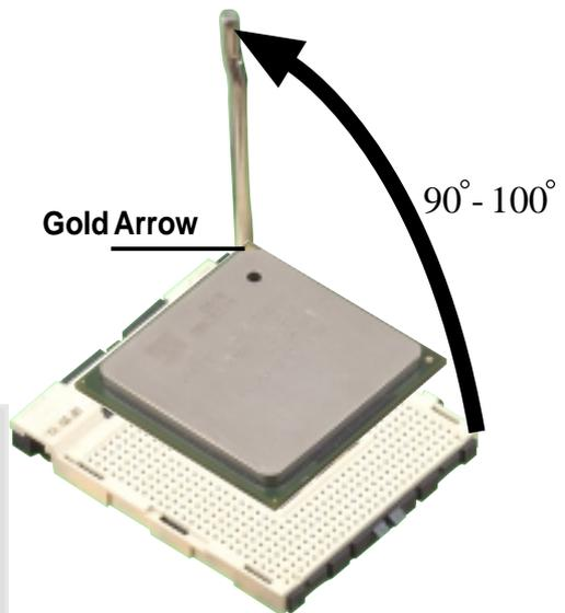
3. Once completely inserted, press the CPU firmly and close the socket lever until it snaps into its locked position.
