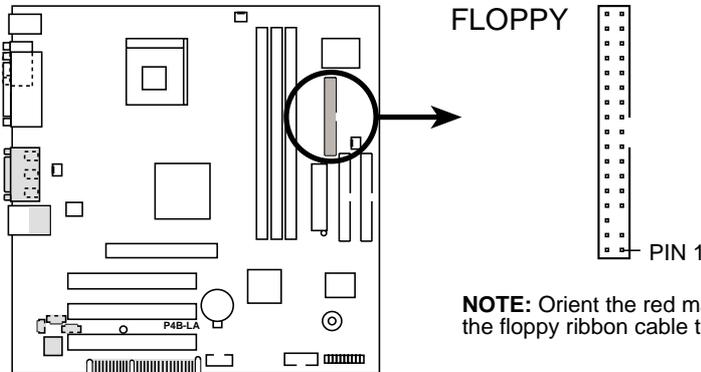
**NOTE:** Orient the red markings on the floppy ribbon cable to PIN 1.
