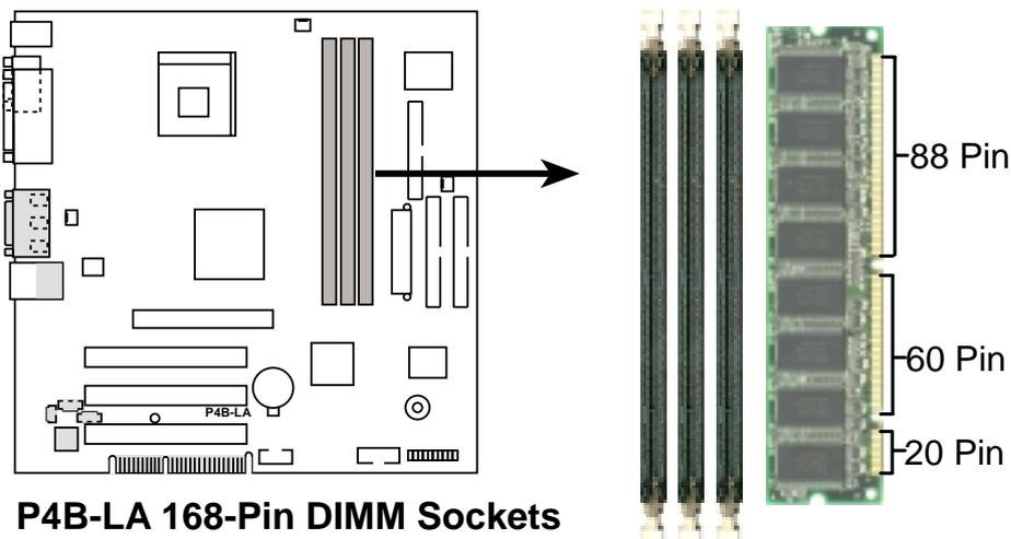
The DIMMs must be 3.3Volt unbuffered SDRAMs. To determine the DIMM type, check the notches on the DIMMs (see figure below).
