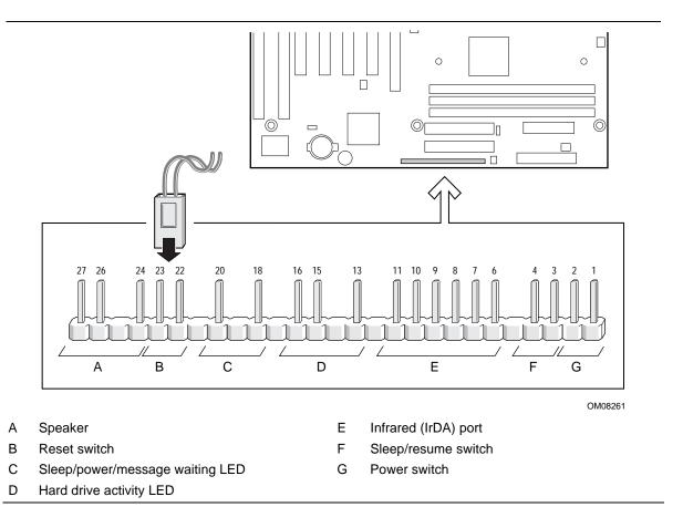
Figure 5. Front Panel I/O Connectors
