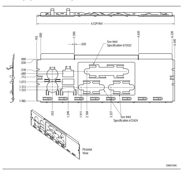
Figure 3. Back Panel I/O Shield Dimensions (ATX Chassis-Dependent)
