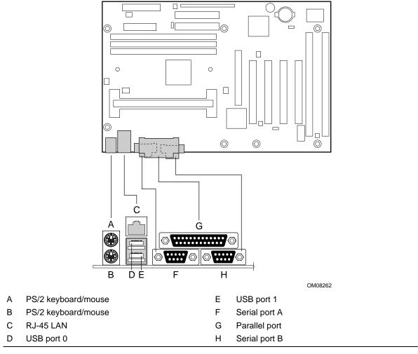
Figure 6. Back Panel I/O Connectors
