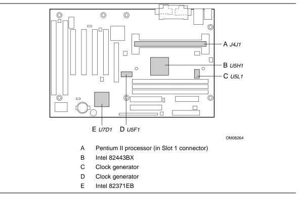
Figure 8. Thermally-Sensitive Components
