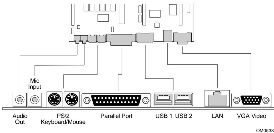
**Figure 5. I/O Connections**
