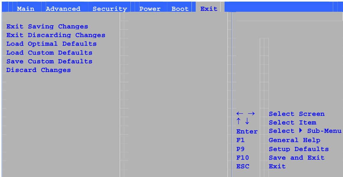
The menu shown in Table 37 is used to exit the BIOS Setup program, saving changes, and loading and saving defaults.
