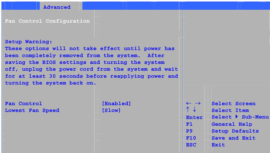
The menu shown in Table 27 is used to configure hardware management features.
