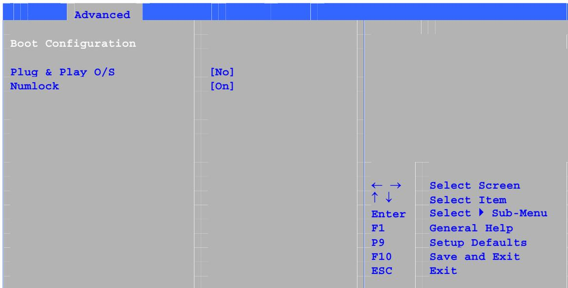
The submenu shown in Table 18 is used to set the Plug & Play options and the power-on state of the Numlock key.
