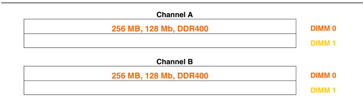
**Figure 8. Dual Configuration Example with Two DIMMs**
