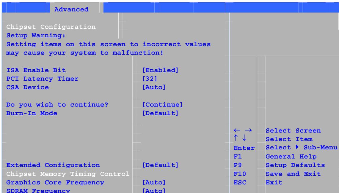
The submenu shown in Table 26 is used to configure advanced chipset features.
