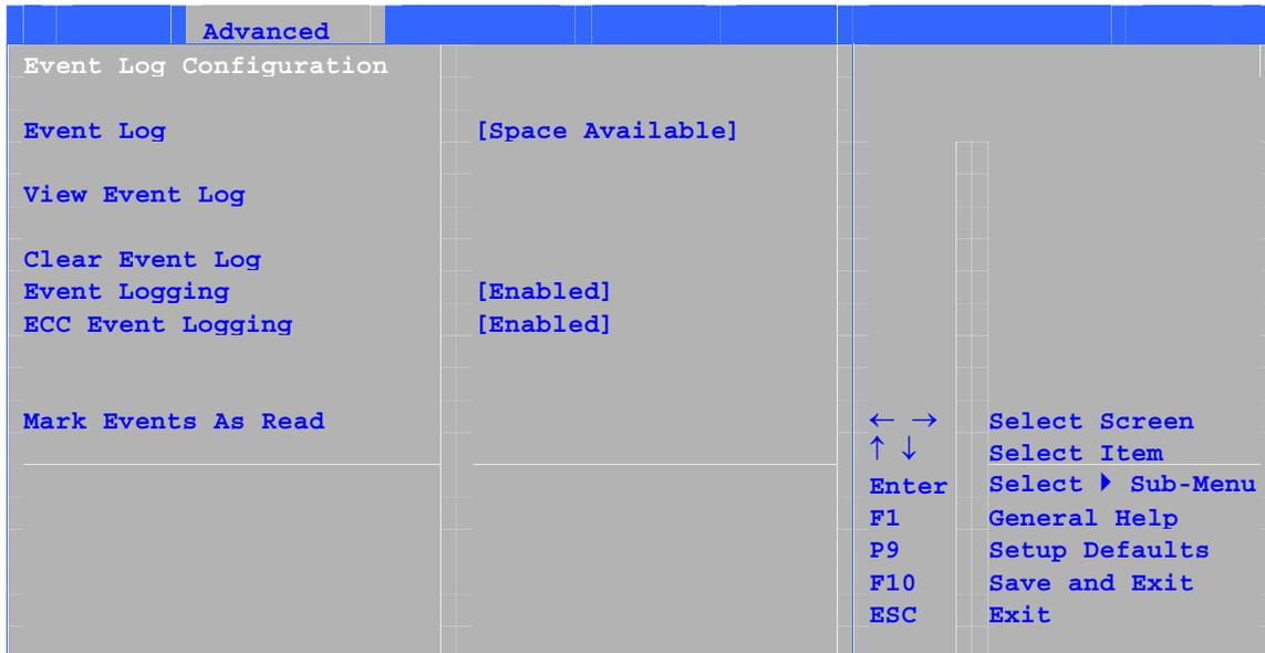
The submenu shown in Table 23 is used to configure the event logging features.
