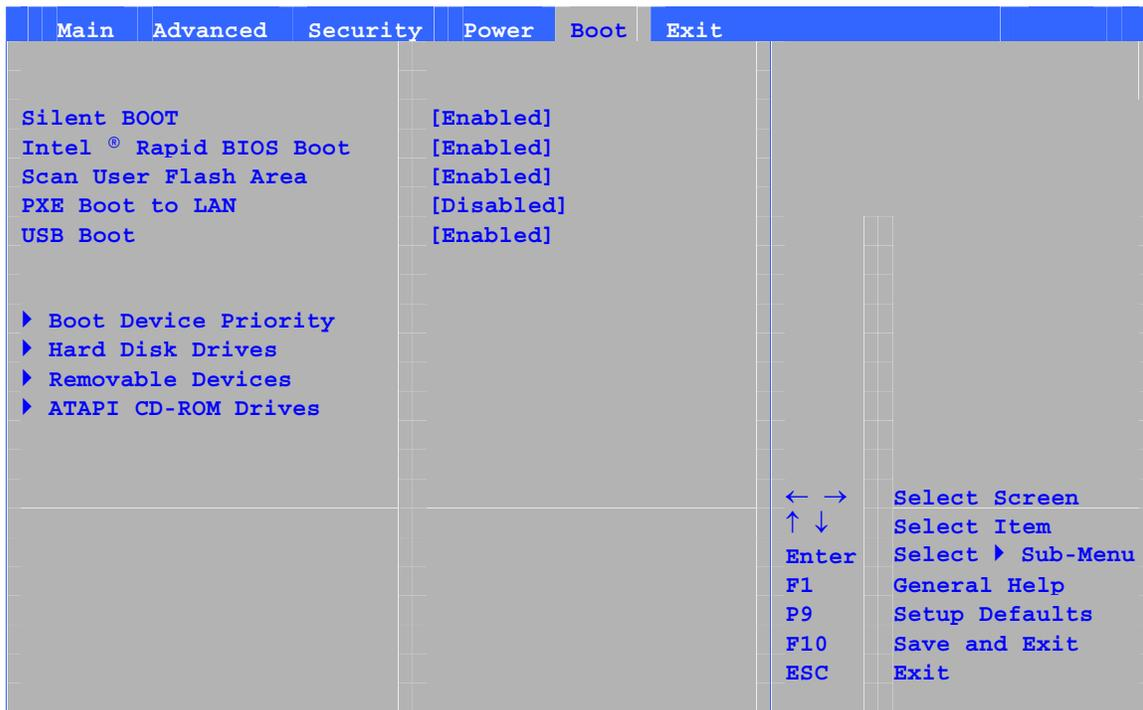
The menu shown in Table 32 is used to set the boot features and the boot sequence.
