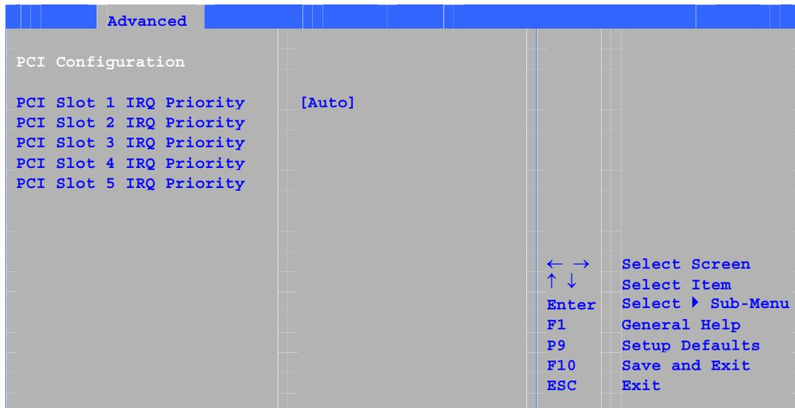
The submenu shown in Table 17 is used to configure the IRQ priority of PCI slots individually.
