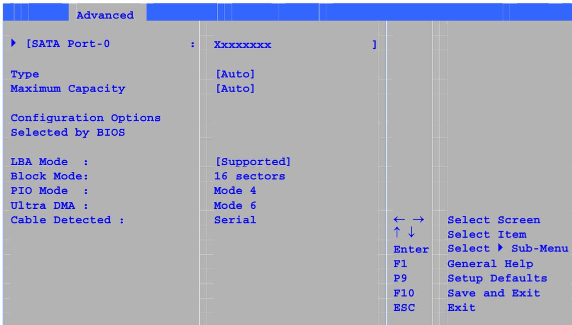
There are four IDE submenus: Primary master, primary slave, secondary master, and secondary slave. Table 21 shows the format of these IDE submenus. For brevity, only one example is shown.
