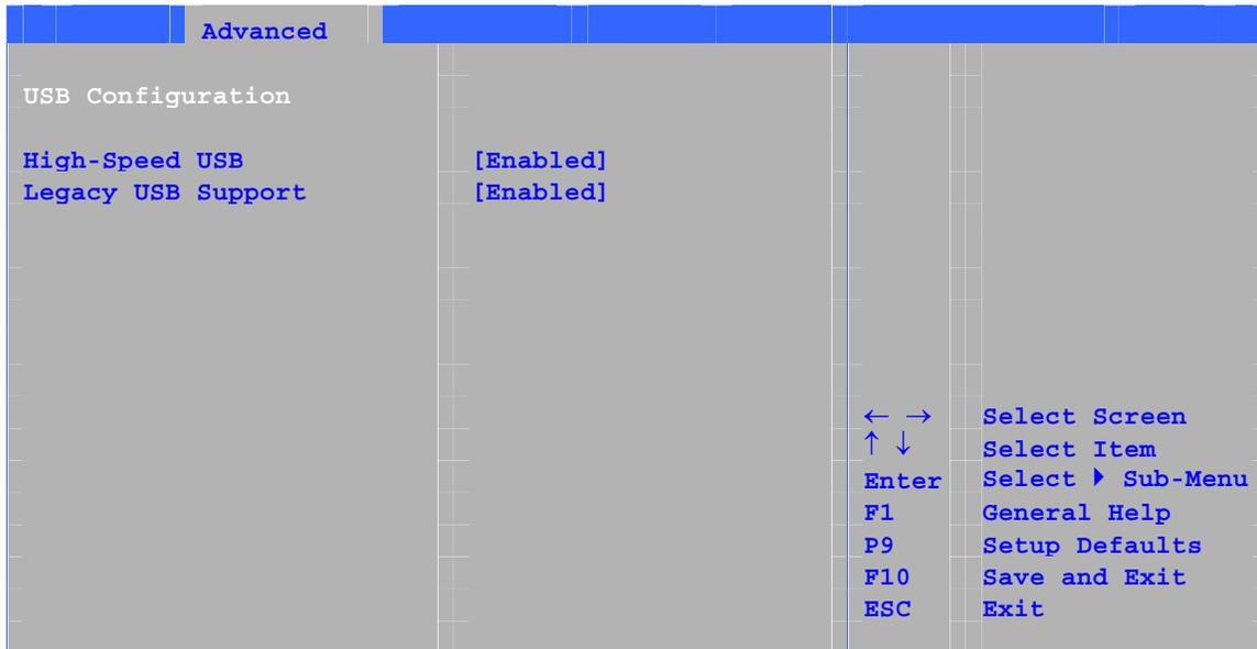
The submenu shown in Table 25 is used to configure USB features.
