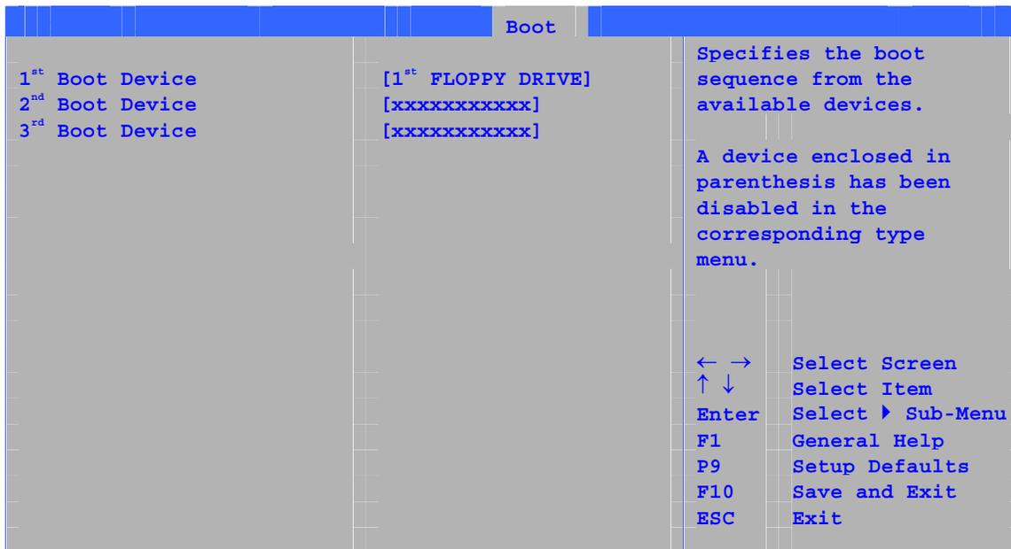
The submenu represented in Table 33 is for setting boot devices priority.
