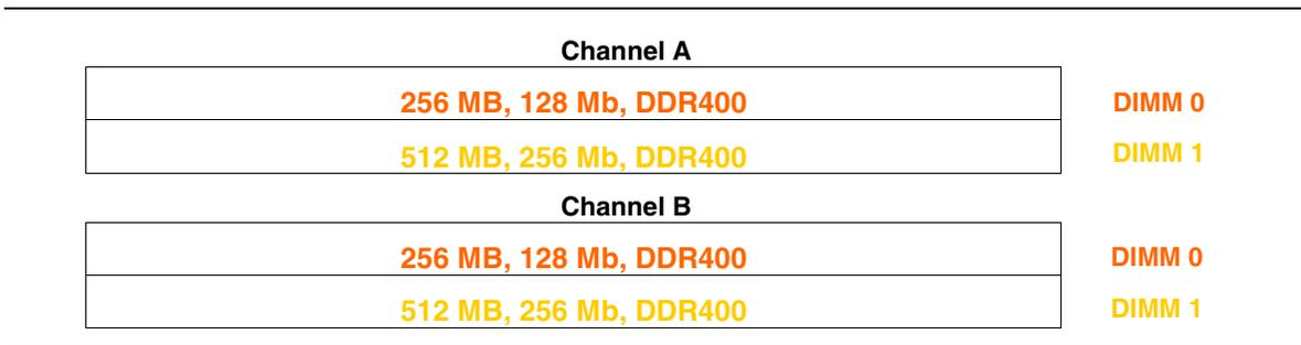
**Figure 9. Dual Configuration Example with Four DIMMs**
