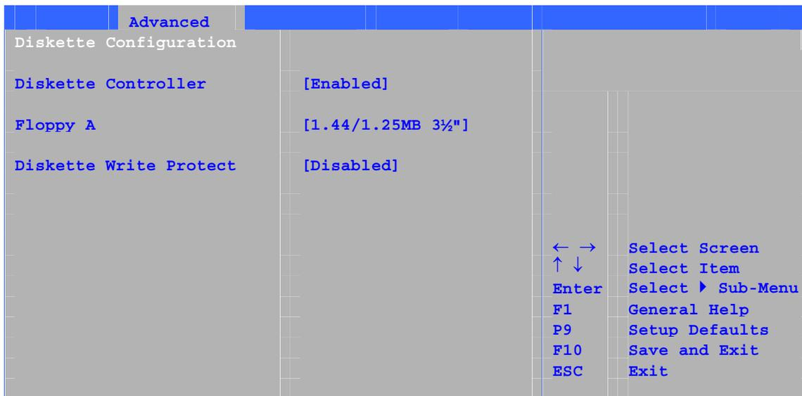
This submenu shown in Table 22 is used to configure the floppy drive.
