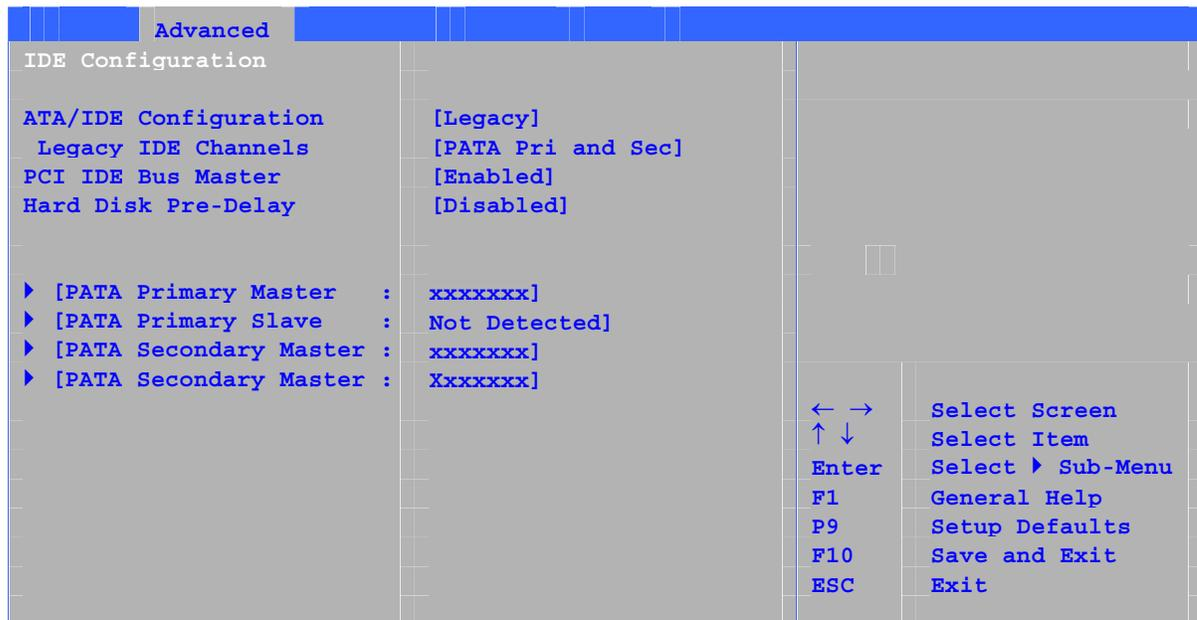
This submenu shown in Table 20 is used to configure IDE device options.
