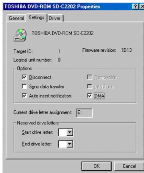
**Figure 2: Checking for DMA**
