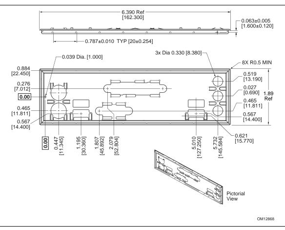
Figure 20. I/O Shield Dimensions (for Desktop Boards with no LAN Subsystem)
