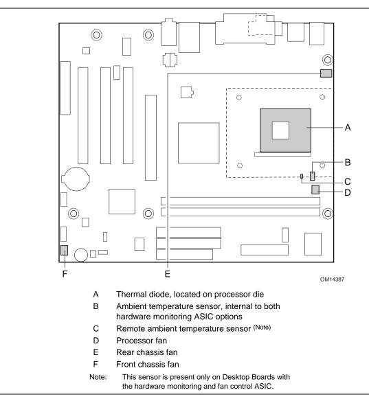
Figure 8. Thermal Monitoring
