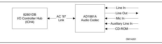
Figure 6. Audio Subsystem Block Diagram
