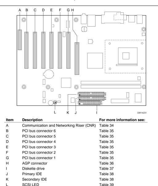
Figure 13. D845EBG2 Add-in Board and Peripheral Interface Connectors
