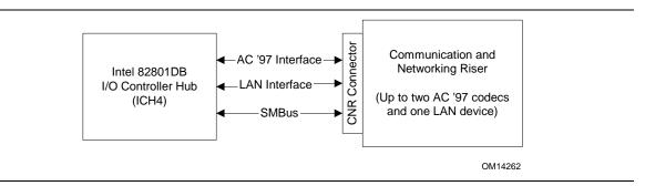
Figure 7. ICH4 and CNR Signal Interface
