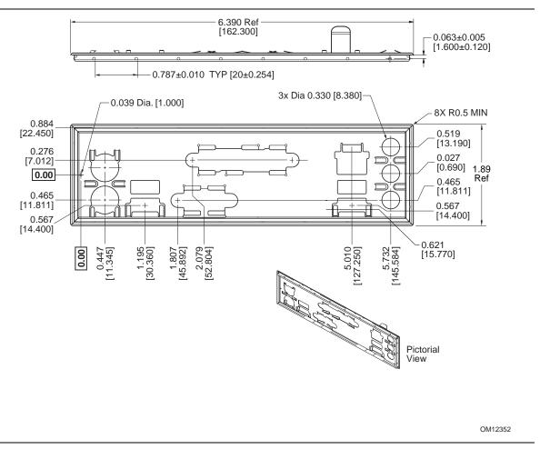
Figure 19. I/O Shield Dimensions (for Desktop Boards with the LAN Subsystem)
