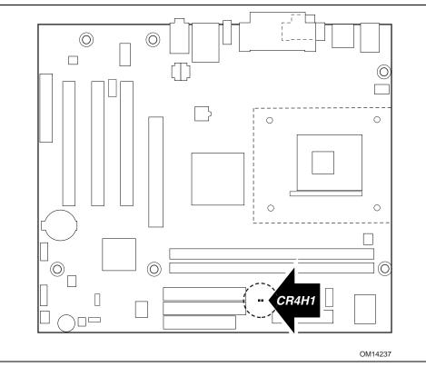
Figure 9. Location of the Standby Power Indicator LED
