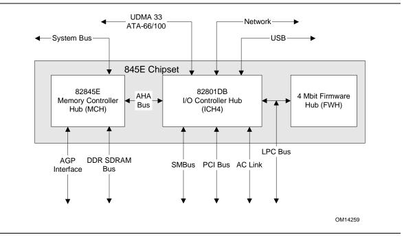
Figure 4. Intel 845E Chipset Block Diagram
