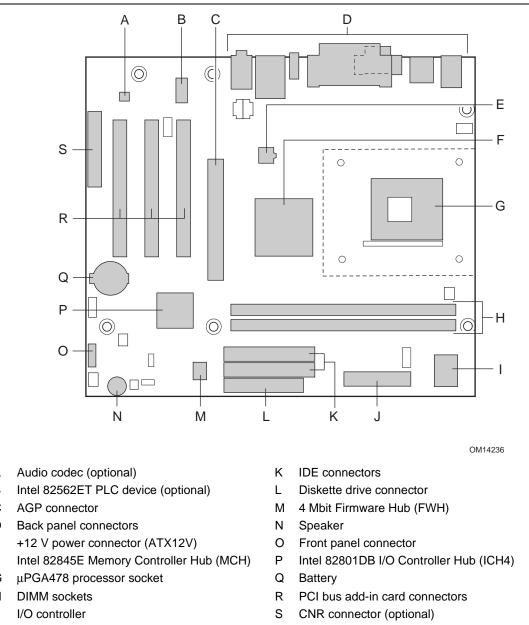
Figure 2 shows the location of the major components on the Desktop Board D845EPT2.
