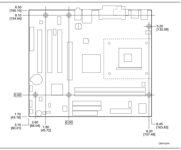
Figure 18. Desktop Board D845EPT2 Dimensions
