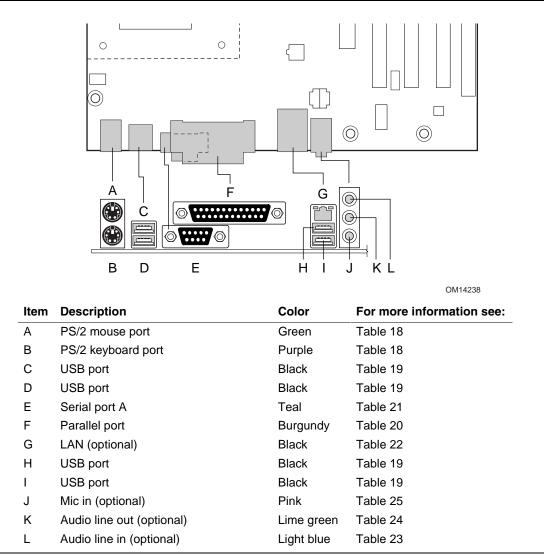
Figure 10. Back Panel Connectors
