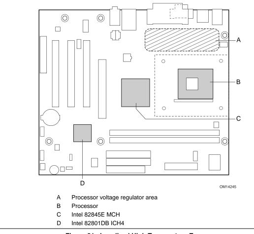
Figure 21 shows the locations of the localized high temperature zones.
