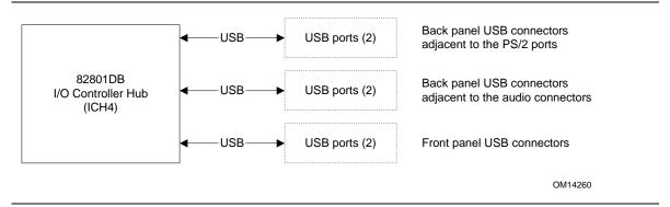
Figure 5. USB Port Configuration
