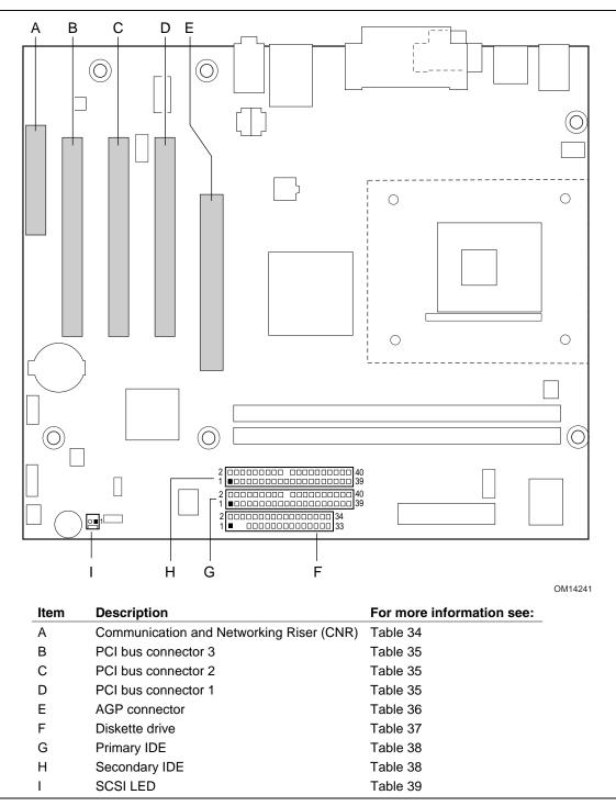
Figure 14. D845EPT2 Add-in Board and Peripheral Interface Connectors
