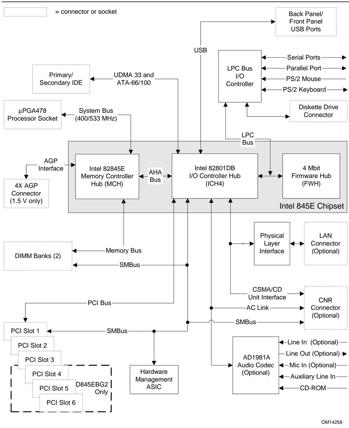
Figure 3. Block Diagram
