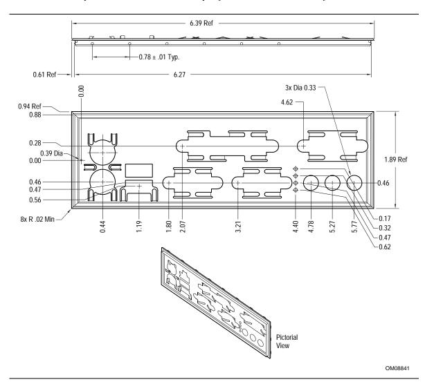
Figure 17. I/O Shield Dimensions (for CC820 Boards with Audio Connectors)
