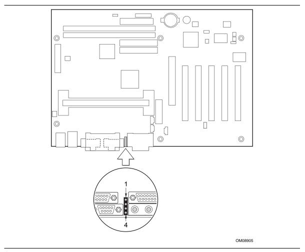
Figure 21. Enhanced Diagnostic LEDs
