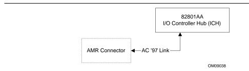
Figure 4. Block Diagram of Audio Subsystem (with ICH and AMR)
