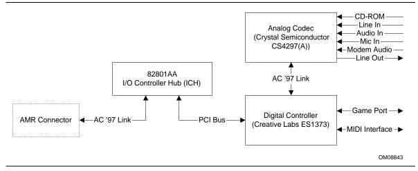
Figure 5. Block Diagram of Audio Subsystem with Analog Codec and Digital Controller
