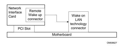
Figure 6. Using the Wake on LAN Technology Connector
