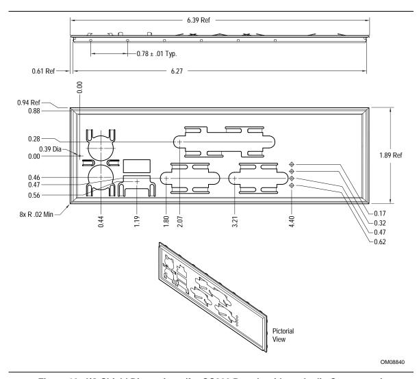
Figure 18. I/O Shield Dimensions (for CC820 Boards without Audio Connectors)
