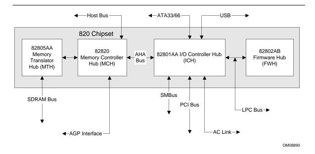
Figure 3. Intel 820 Chipset Block Diagram
