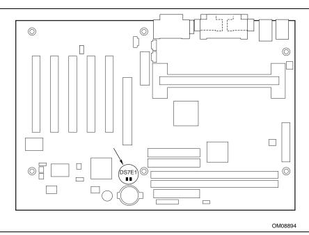
Figure 7. Location of Standby Power Indicator LED
