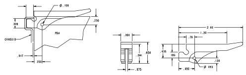
Figure 5.4 Module Insertion/Extractor Handle
