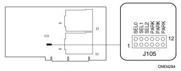
**Figure 1.20 Processor Frequency Jumpers**
