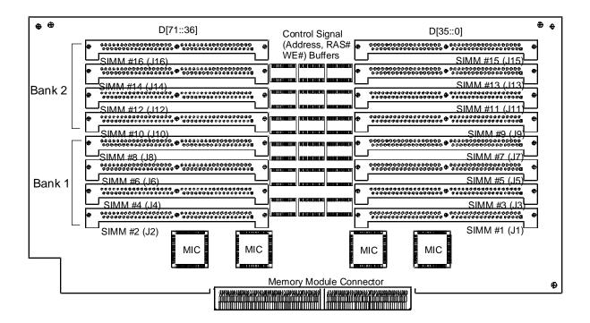
Figure 1.5 1GB Memory Module Layout
