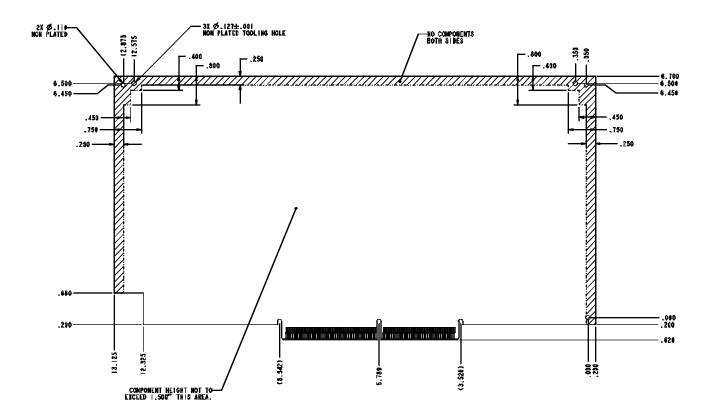
**Figure 5.2 Memory Module Mechanical Specifications**
