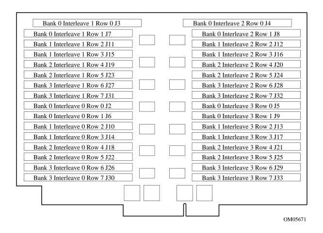
Figure 1.6 4GB Memory Module Layout
