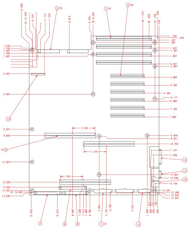
Figure 5.3 Baseboard Mechanical Specifications
