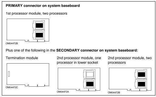
**Figure 1.9 Processor Configuration Models**
