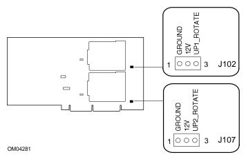
Figure 1.21 Fan Sink Connectors
