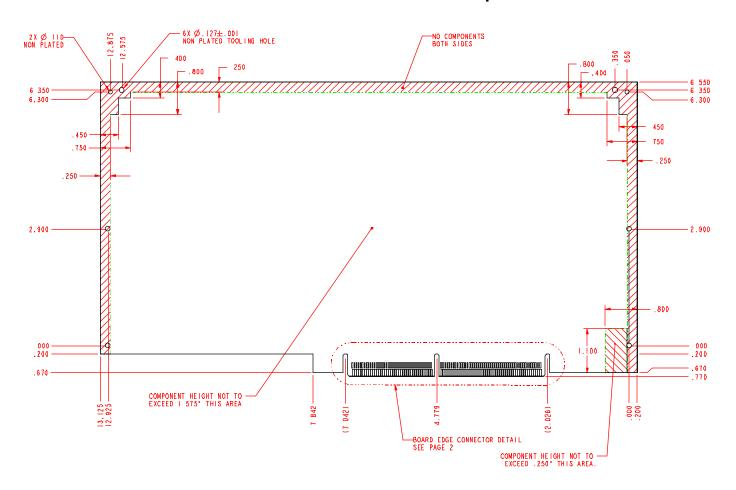
Figure 5.1 Processor and Terminator Module Mechanical Specifications
