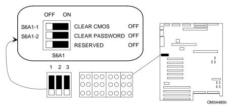
Figure 1.17 Clear CMOS/Password Switch
