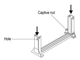
5. Tighten the captive nuts to stabilize the Retention Mechanism.
