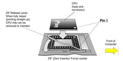
**Inserting a CPU**
