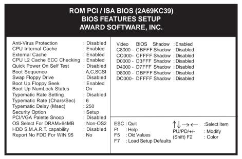
Figure 3-3 BIOS Feature Setup Screen
