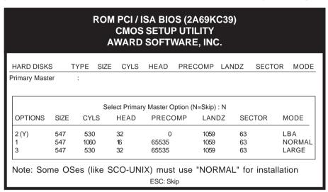
Figure 3-12 IDE HDD Auto Detection Screen
