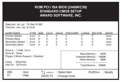
Figure 3-2 Standard CMOS Setup Screen
