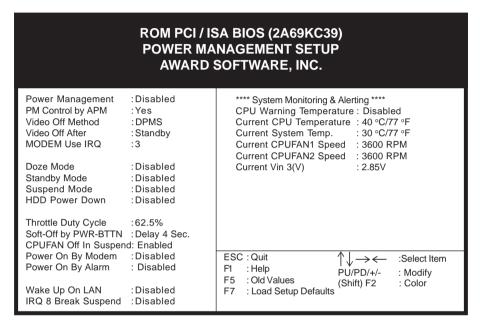
Figure 3-5 Power Management Setup Screen
