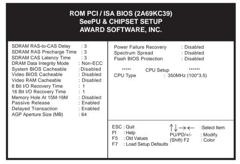
Figure 3-4 Chipset Features Setup Screen
