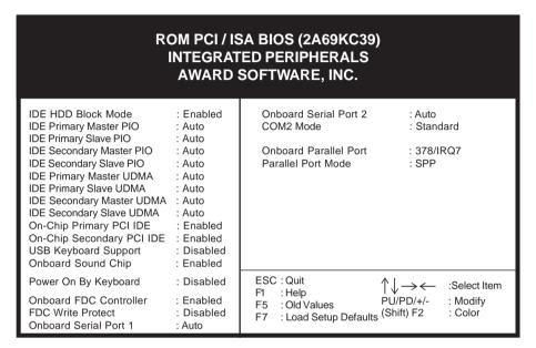
Figure 3-9 Integrated Peripherals Setup Screen
