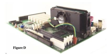
Figure D above shows a properly installed SECC2 CPU using the retention module. Note the direction of the CPU fan and the way in which the cable is connected.
