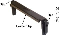
Make sure the lower lip of the overhead clip is oriented towards the opposite side of the CPU fan (see Figure I left).
