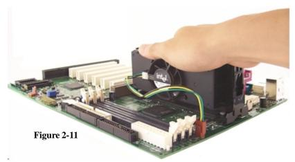
Line up the retention brace with the holes provided on the motherboard. At the same time, make sure the CPU is lined up with the CPU slot. Lower the CPU onto the motherboard. The mountings on the retention brace should fit through the holes of the motherboard and the CPU should fit into the slot. (See Figure 2-11). Secure the retention brace. The end result should look like Figure 2-12.
