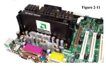
You will also need to connect the CPU's cooling fan cable to the cooling fan power connector on the board. Locate the cooling fan connector (e.g. FAN1) on the motherboard. Plug the CPU's cooling fan cable into the cooling fan
