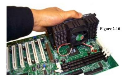
Carefully line up the pins of the CPU with the pins of the Slot while placing the CPU between the two retention braces (the CPU cooling fan should face the memory DIMM sockets). Lower the CPU onto the motherboard (see Figure 2-10 above). Your CPU will be firmly secured onto the motherboard once the retention braces "snap" into the sides of the CPU. The installed CPU should look like Figure 2-11 below.
