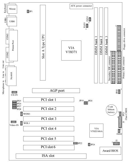
The tiny "1"s next to jumpers of 3 pins or more indicate the position of pin 1 for that jumper.
