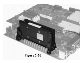
When removing the CPU, unscrew the nuts on the retention braces and remove all three components at once. This may require careful firm tugs to pull the CPU out of its slot.
