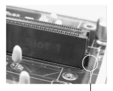
Figure 2-8 - Pentium II Slot Connector and Key Pin
