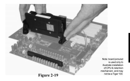
Be sure to line up the holes of the retention brace with the screws protruding from the motherboard. At the same time, make sure the CPU is lined up with the CPU slot. Lower the three components onto the motherboard. The screws on the motherboard should fit through the holes of the retention braces and the CPU should fit into the slot. Secure the retention braces with the nuts provided in the package. The end result should look like Figure 2-20.
