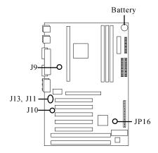
connectors is directed through the Ensoniq 1371 PCI sound chip, and the digital signal is turned into an audio signal which goes out through the speaker. The TDA connector (J10) is for modem audio; the MPEG connector (J9) is for DVD and TV cards; the VIDEO connector is (J11); the CD connector (J13) is for CD-ROMs.
