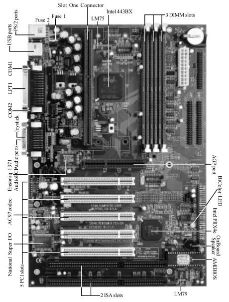
F1 (Fuse 1), F2 (Fuse 2): Rated 30V DC, hold current at 1.6 A.
