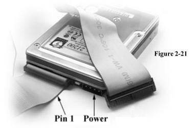
In most cases, this is the proper way of connecting your IDE cable to the harddrive. Figure 2-22 on the following page shows the IDE cable properly connected to the motherboard. Contact your hard disk drive manufacturer or documentation for more information.
