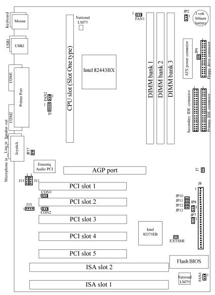
The tiny "1"s next to jumpers of 3 pins or more indicate the position of pin 1 for that jumper.
