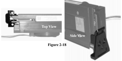
When both braces are properly positioned, press both braces against the sides of the CPU and carefully lift them over the CPU slot on the motherboard. Warning - Because the braces are loosely held against the CPU, they can easily fall off. You must hold both braces against the CPU while lifting all three components above the motherboard. (See Figure 2-19 on the following page.)
