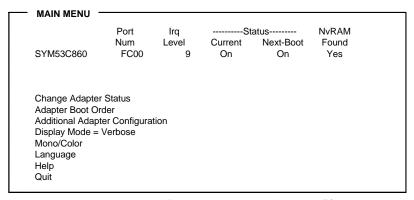
You can select an adapter only if the current status is On. Changes are only possible with SCSI adapters that support NVRAM (non-volatile memory). Check the NvRAM Found column to see if NVRAM is present on your adapter. If you choose to alter any of these settings, exit via the Quit option and the system will reboot.
