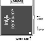
a white dot on top of the CPU. Align this corner towards the end of the lever as shown in the figure below. Insert the CPU, hold it down, and close the lever until it locks into place.
