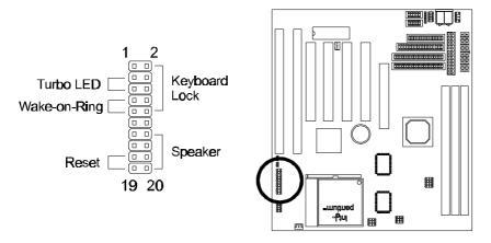
**Pins [3 & 5] Turbo LED switch** - The Turbo function is not supported by this mainboard. Therefore, the Turbo LED will always remain lit as long as the system power is on.
