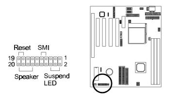
**Pins [7 & 9] SMI suspend switch lead** - If your system's case has a suspend switch, hook the lead from the switch to pins 7 & 9. A suspend switch is used to save electricity by putting the system into a suspend mode when the computer is not being used. For this switch to be functional, "*Suspend Mode*" must first be enabled in the **Power Management Setup** in the BIOS Setup utility.
