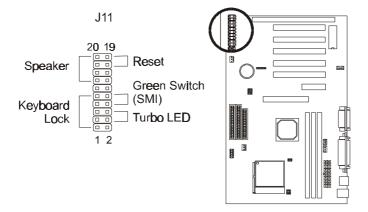
**Pins [3 & 5] Turbo LED lead** – The Turbo function is not supported by this mainboard. Therefore, the Turbo LED will always remain lit as long as the system power is on.
