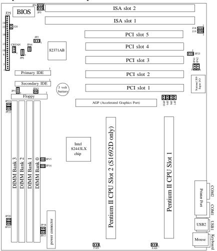
The tiny "1"s next to jumpers of 3 pins or more indicate the position of pin 1 for that jumper. Refer to pages 14-16 for the jumper and pin assignments.
