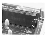
Pentium II Slot Connector and Key Pin
