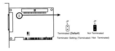
Decide whether or not you need to terminate the ASUS PCI-SC200 based on its position in the SCSI chain. Only the devices at each end of the chain need to be terminated. If you have **only** internal or **only** external devices connected to the ASUS PCI-SC200, then you **must** terminate the ASUS PCI-SC200. If you have **both** internal and external devices connected, you **must not** terminate the card. See the following example which illustrates this concept.
