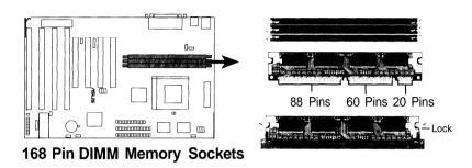
The Dual Inline Memory Module (DIMM) memory modules must be 3.3Volt Unbuffered Synchronous DRAM (SDRAM) or Extended Data Output (EDO). You can identify the type of DIMM module by the illustration below:
