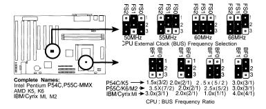
Set the jumpers by the Internal speed of the Intel, AMD, IBM, or Cyrix CPU as follows:
