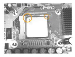
Step 3 : Push the lever down to close the socket.
