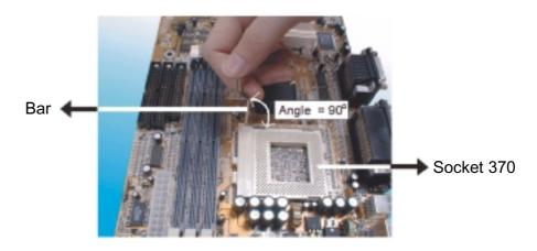
3. Locate Pin 1 in the socket and look for the cut edge in the CPU, match Pin 1 with the cut edge then insert the CPU. It should be inserted easily.
