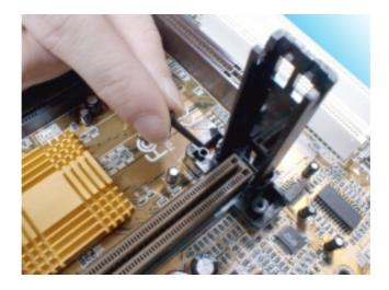
5. Slide the CPU slowly into Slot1 along the two sides of the CPU Retention.
