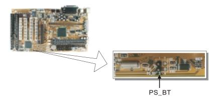
In Windows 98/95, under the "SHUT DOWN" option, the computer's power will switch off automatically and put the PC in a suspend mode. A blinking power light will indicate this. To restart the system, simply press the Power Button.
