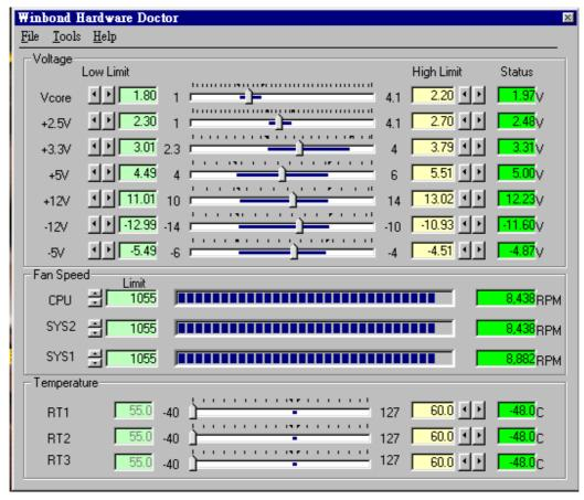
The Application of W83781D also controls the fan speed. The default of CPU Fan, SYS1 Fan and SYS2 Fan is "Enable".
