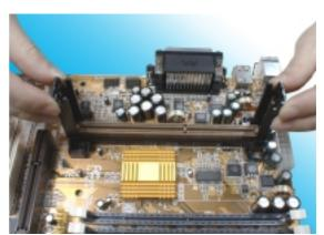
4. Ensure that the CPU Retention has been slotted all the way in, then screw the four plastic screws into the sockets on each side of Slot1 to make sure that the CPU Retention is fixed firmly in position.
