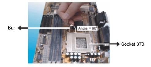
3. Locate Pin 1 in the socket and look for the cut edge in the CPU, match Pin 1 with the cut edge then insert the CPU. It should insert easily.
