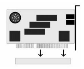
Figure 3-5: Installing an ISA Peripheral Card
