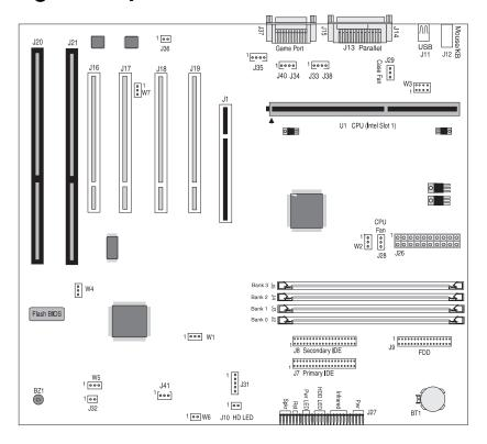
Figure 2-1: Tigercat System Board Diagram
