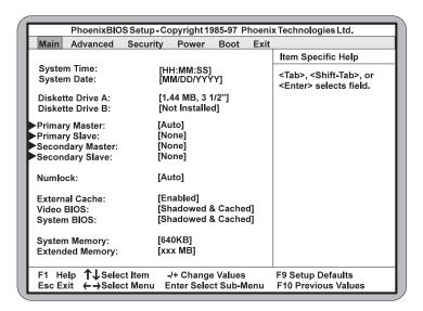
Figure 4-2: CMOS Main Screen
