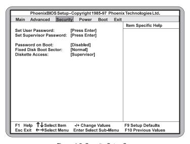
Figure 4-5: Security Setup Screen
