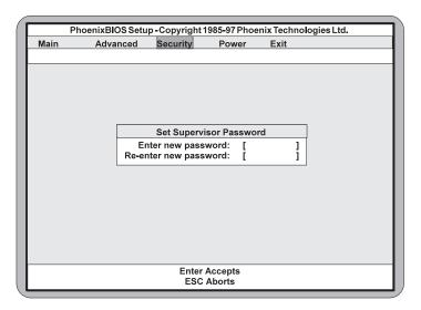
Figure 4-6: Supervisor Password Submenu
