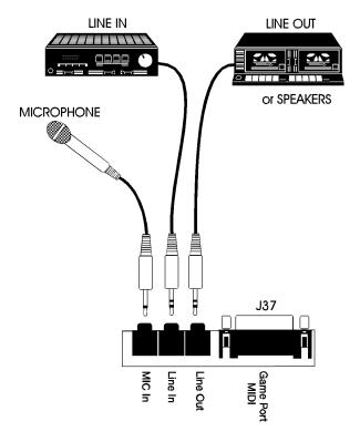
Figure 3-7: Connecting External Sound Devices
