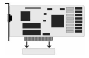
Figure 3-4: Installing a PCI Card
