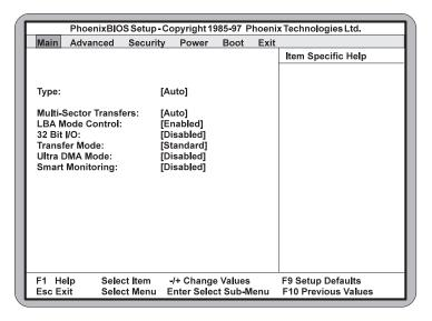
Figure 4-3: IDE Device Submenu
