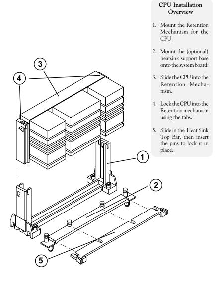
Figure 3-2: Installing a CPU
