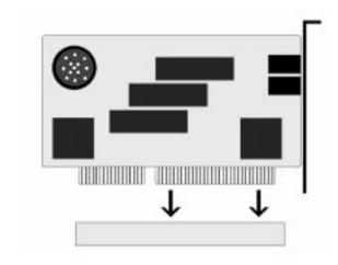
Figure 3-5: Installing an ISA Peripheral Card
