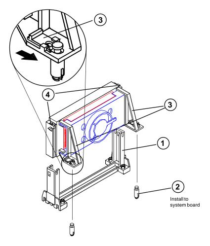
Figure 3-3: Installing a CPU (Boxed version)
