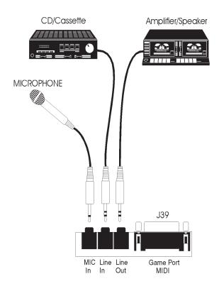
Figure 3-6: Connecting External Sound Devices
