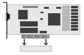
Figure 3-4: Installing a PCI Card
