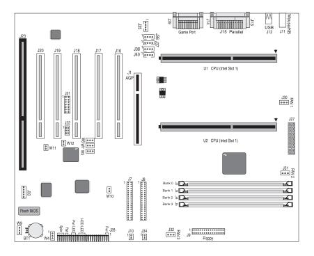
Figure 2-1: Helios System Board Diagram
