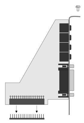
Figure 3-3 Installing the Sound Riser Card
