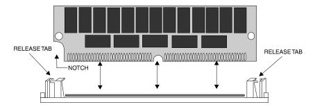
Figure 3-1 Installing a 72-Pin SIMM
