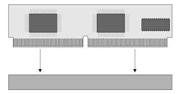
Figure 3-2 Installing a Cache Module
