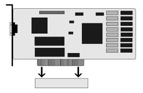
Figure 3-5 Installing a PCI Peripheral Card
