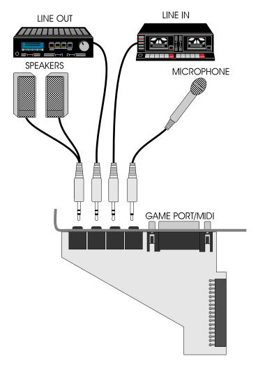
Figure 3-4 Connecting External Devices to the Sound Controller
