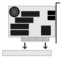
Figure 3-6 Installing an ISA Peripheral Card
