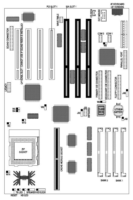
Figure 2-1 M54Hi-Plus System Board
