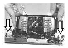
Step 3: Pull the clip beside retention mechanism upward to lock the CPU.
