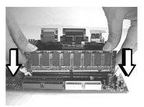
Step 3: Press the latches into the notches of the RAM module
