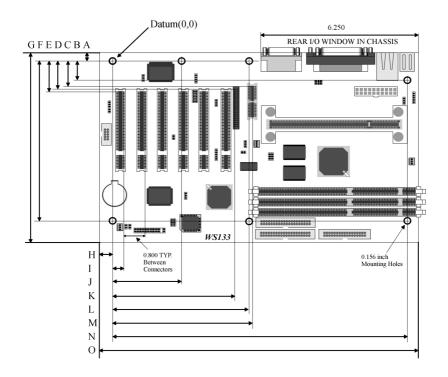
A:0.400 inch B:0.900 inch C:1.060 inch D:1.085 inch E:1.225 inch F:6.100 inch G:7.402 inch H:0.650 inch I:0.310 inch J: 3.100 inch K:4.482 inch L:4.900 inch M:5.012 inch N:11.100 inch O:12.000 inch
