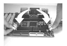
**Step 2:**Insert the RAM module into the DIMM Secket
