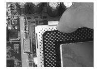
**Step4:** Push the lever down to close the socket.
