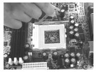
**Step2:** Insert the CPU into the socket. Please keep the lever right angle when inserting CPU.
