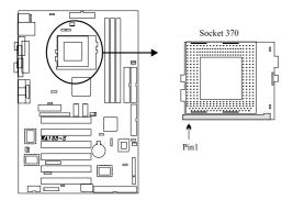
**Step1:** Locate the ZIF socket and open it by first pulling the lever of socket upward.
