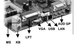
(burgundy), which is J33 on the motherboard. Then, connect your parallel port device to the parallel port connector.
