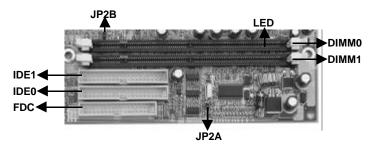
**Warning:** In order to support the latest STR (Suspend to RAM) function, please note that the onboard power supply circuit in memory is independent of all other components. The memory module will always be provided with the necessary current to hold the data stored in memory chips even while the computer has been shut down.
